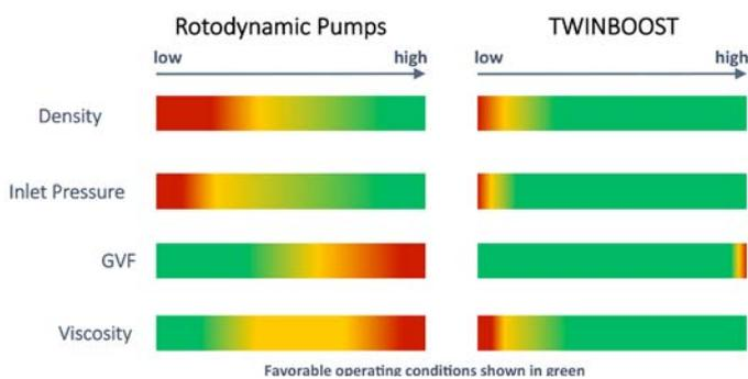
Figure 3. Operating differences TwinBoost and Roto-dynamic technologies.
