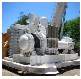
Figure 5. MPAM, retrievable motor pump module.
