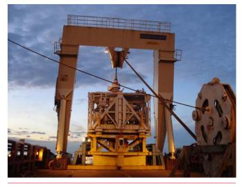
Figure 6. Subsea deployment using anchor handling vessel.
