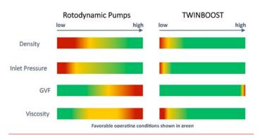
Figure 2. Subsea boosting comparison.
