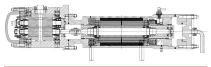
Figure 4. Subsea canned motor-pump.
