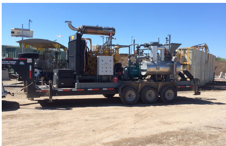
Figure 5. Portable multiphase pump for gas well de-watering.
