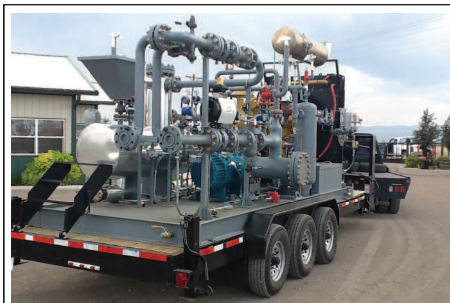
A portable blow-down unit can be towed to the well site by a standard 1.5-ton pickup. The pump is driven by a natural gas engine fueled by gas from the flowline. The unit is equipped with automation, controls and safeties to be completely self-supporting.
