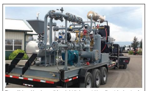
The multiphase blow down unit from Leistritz is a portable, self-contained system for removing liquids and gases from the wellbore while increasing well pressure. Connected to the well's export line, the unit draws down the well's back pressure to increase production stream velocity.
