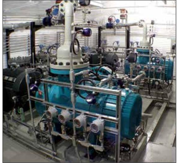
The Leistriz Multiphase Gathering System (MGSs) are expandable versions of the MWS, designed to handle production from multiple wells. Individual MGSs handle total flow rates up to 550,000 bpde and differential pressures up to 1400 psi. These systems are fully automated and can be expanded to operate multiple MGSs in parallel for facilities requiring additional flow capacity.
