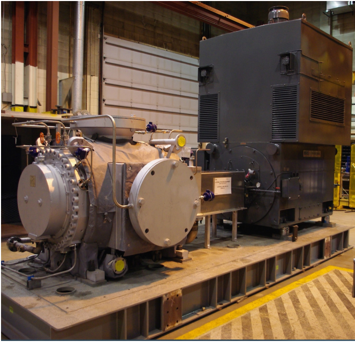
Figure 3. Large twin-screw pump in trunk line service.
