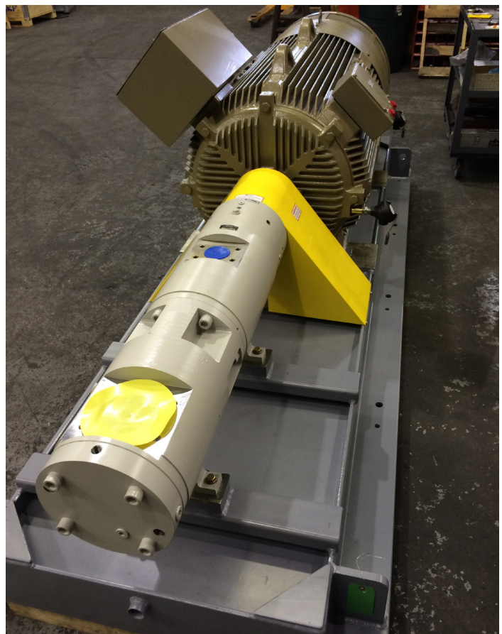
Figure 7. High pressure three-screw pump for light oil and condensate.
